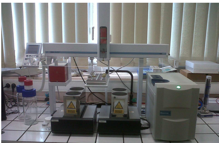
Saint Gobain laboratory, HERACLES electronic nose with 1L vials for incubating large volume sample
