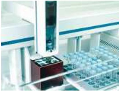
The electronic nose has been found to detect taint in a food packaging board, especially in cases where various autoxidation products (such as hexanal and other aldehydes) have been produced in the paperboard, for example as a result of storage. The nose is also suitable for examining various
